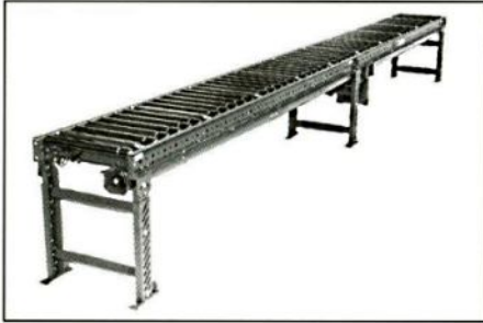
Line shaft zero pressure accumulator
